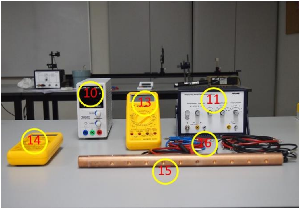
Figure 4. Equipment for the experiment of the electrical conductivity measurements.
