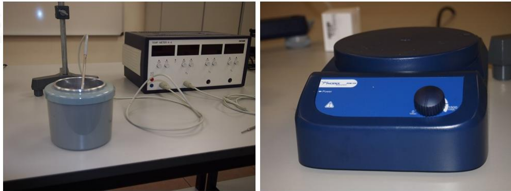
Figure 5. The lower calorimeter and the magnetic stirring. Experimental set up for measuring the influence of the surroundings.
