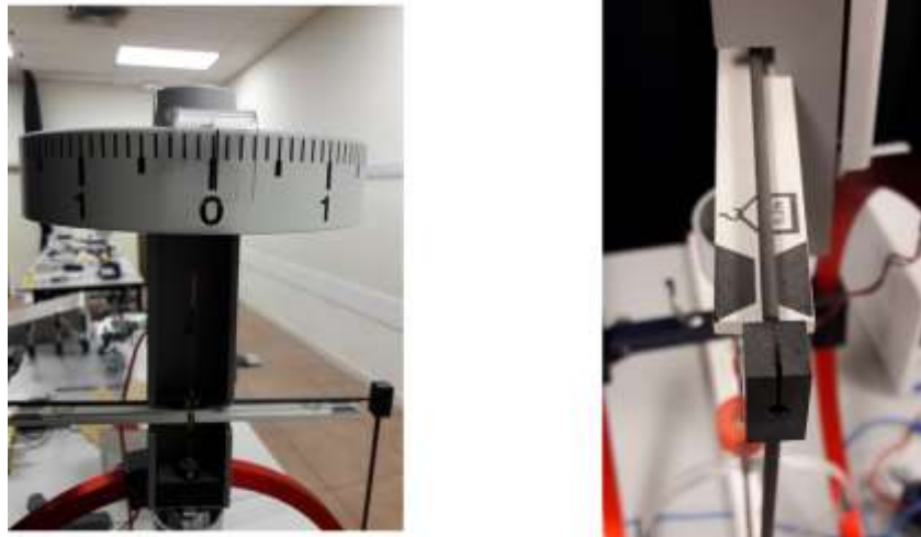
Figure 11: (left) Calibration of the zero force. (right) Lever arm aligned in the middle of the zero mark
